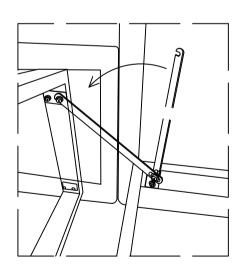
Connect the corner bench and side bench by using the fixing strap. Tighten all the bolts
